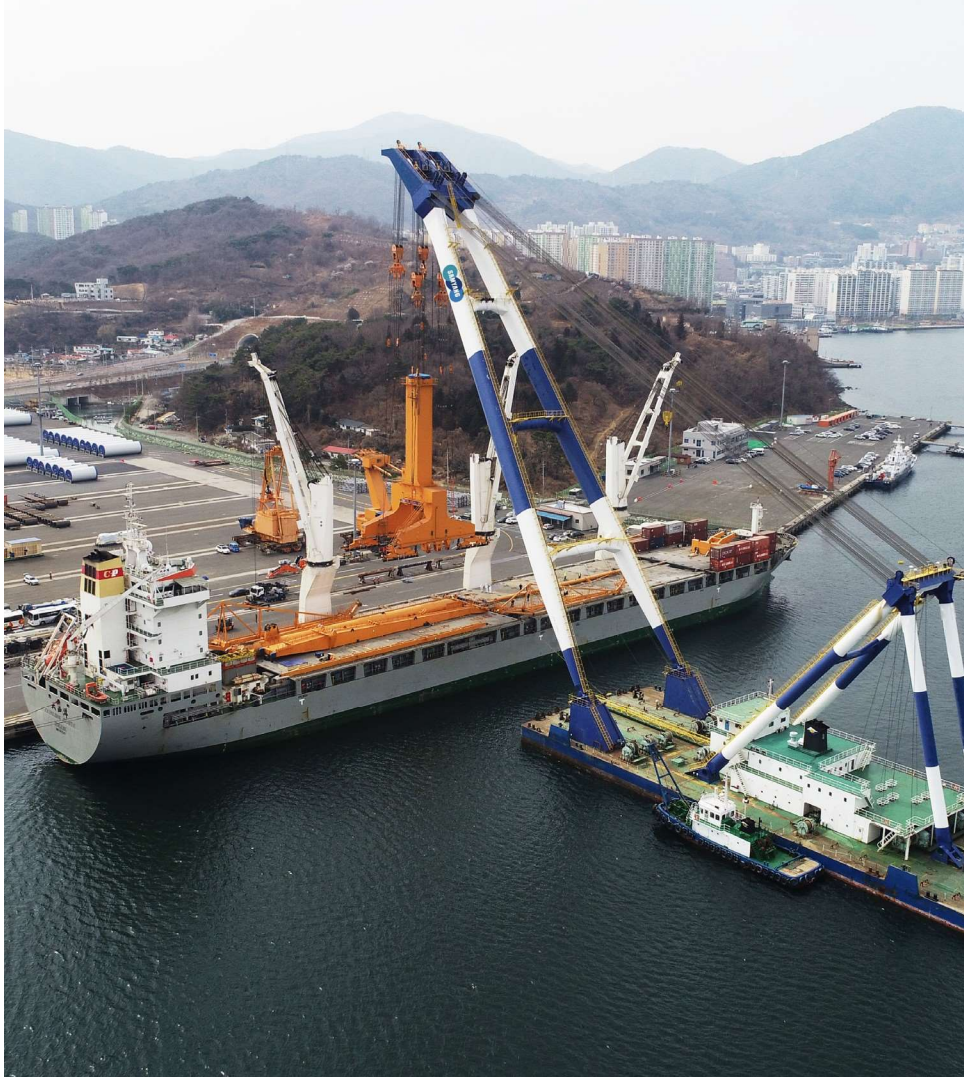
FLOATING CRANE LIFTING CAPACITY S.W.L. : 1,300TONS
